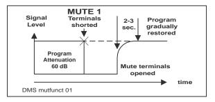
Fig. 17B - M 1 Function Timing Diagram
